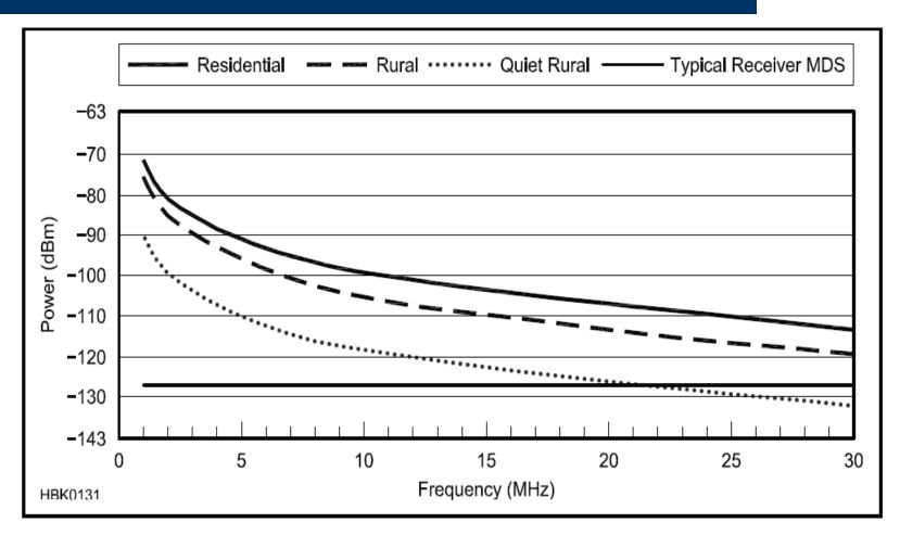
Fig 1 — Typical noise levels versus frequency for various environments. (Manmade noise in a 500-Hz bandwidth, from Rec. ITU-R P.372.7, *Radio Noise*)
