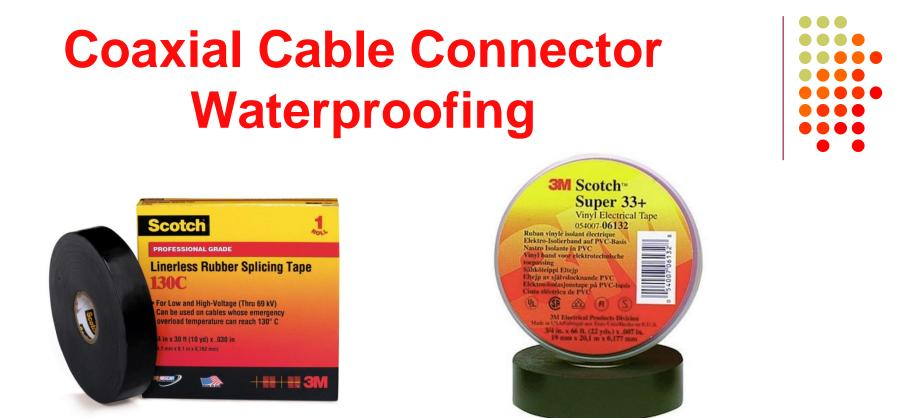
Cover your connectors with two <u>50% overlapped</u> layers of Scotch 130C linerless rubber splicing tape stretched to 50% of its original width, sticky side <u>facing out</u>
